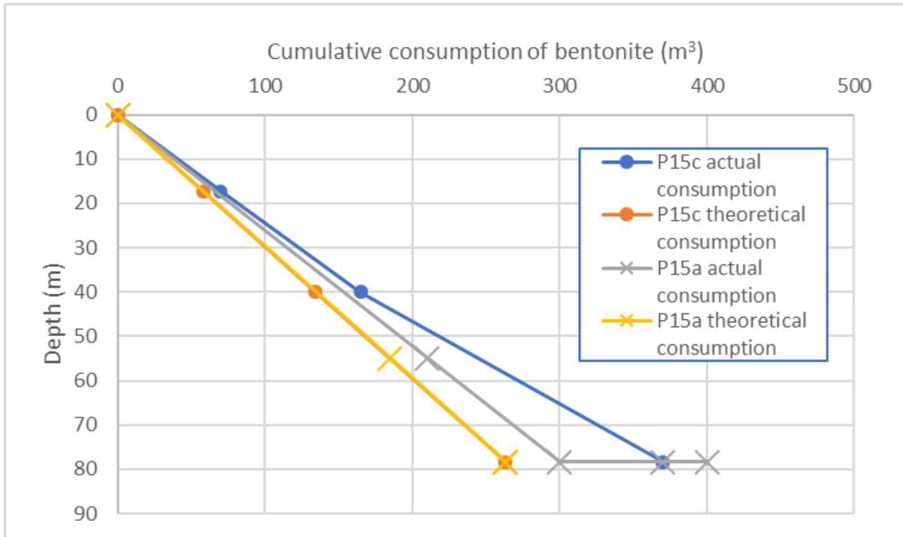
Figure 11 Cumulative consumption of bentonite vs. depth for bites 15a and 15c
