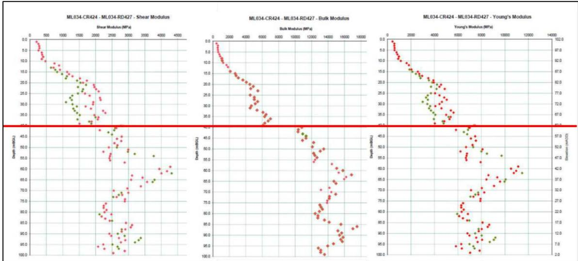
Figure 36 - Cross hole seismic between ML034-RD417 and ML034-CR424
