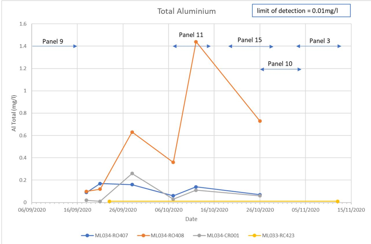
Figure 28 – Total aluminium concentrations during d-walling
