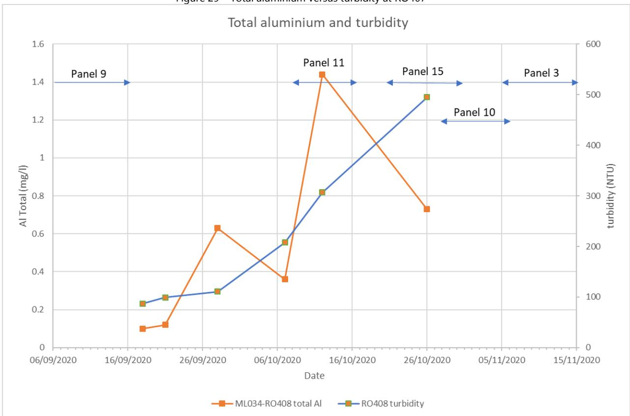
Figure 30 – Total aluminium versus turbidity at RO408
