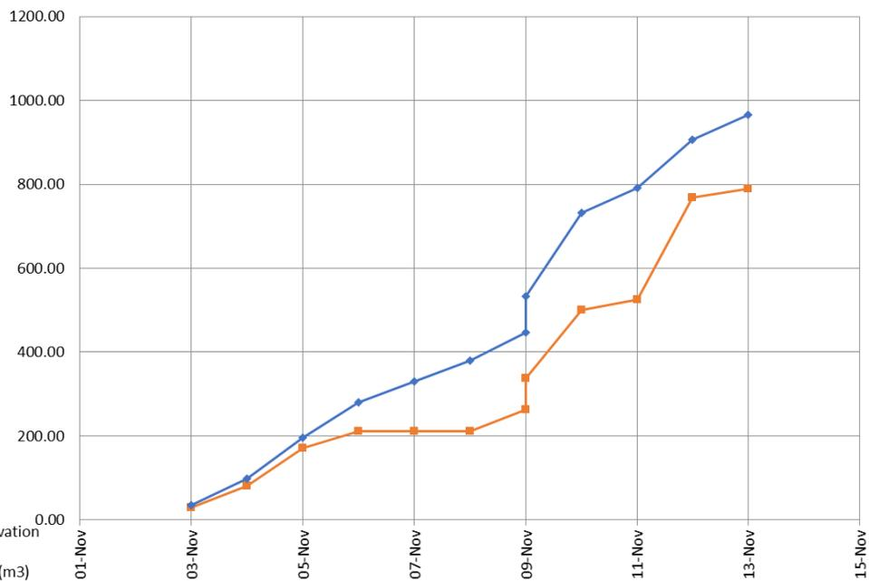
Figure 16 Cumulative consumption of bentonite vs. time for Panel 3
