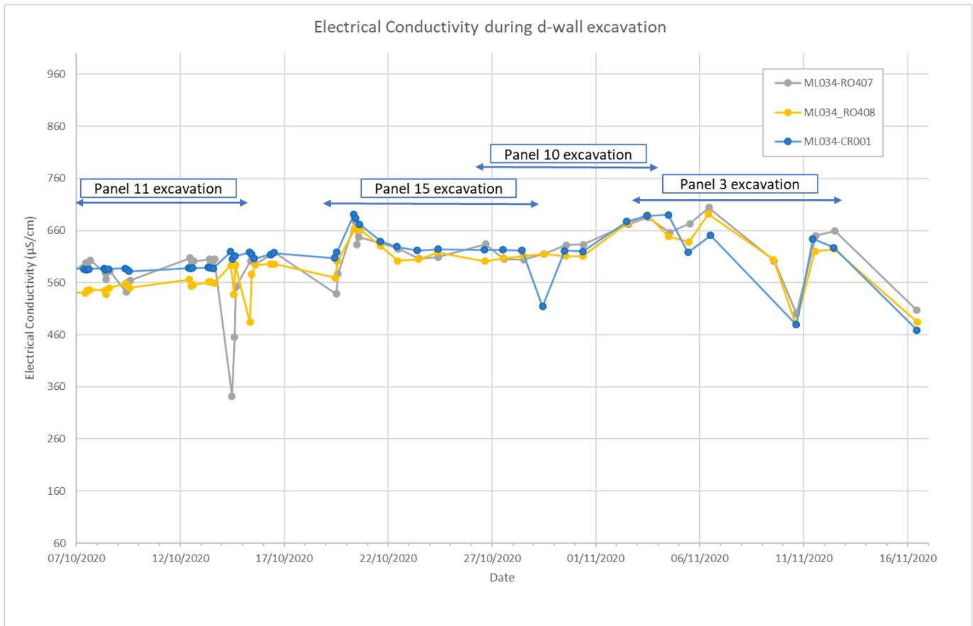
Figure 25 – Electrical conductivity during excavation of Panels 11 to 3
