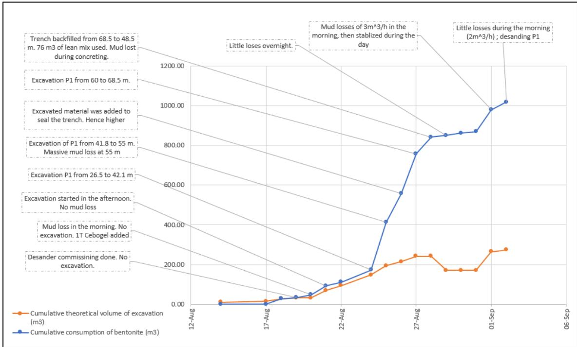
Figure 5 - Cumulative consumption of bentonite vs. time for Panel 1
