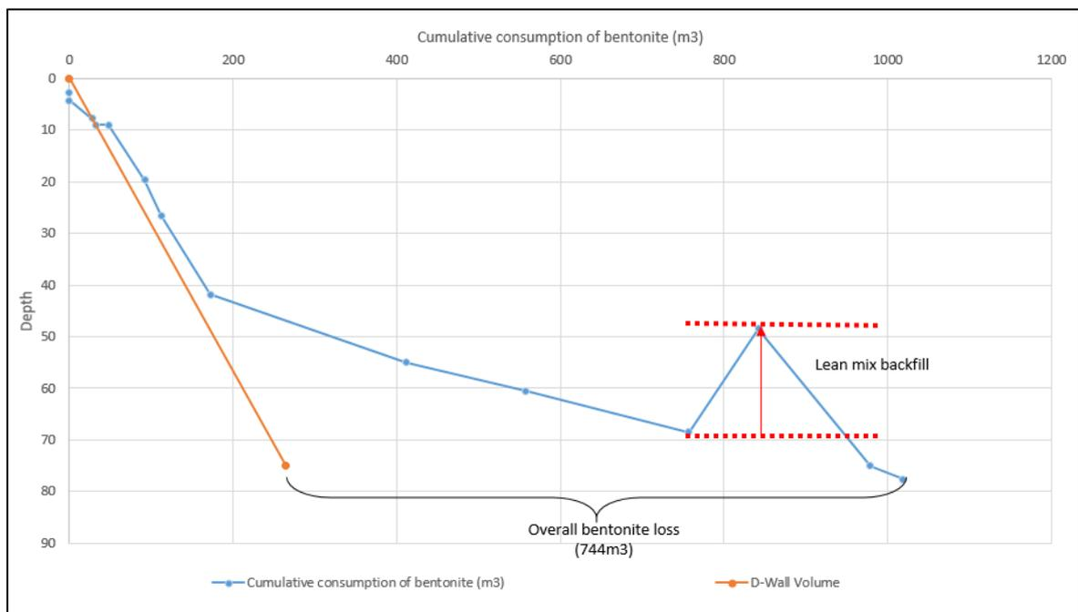
Figure 4 - Cumulative consumption of bentonite vs. depth for Panel 1
