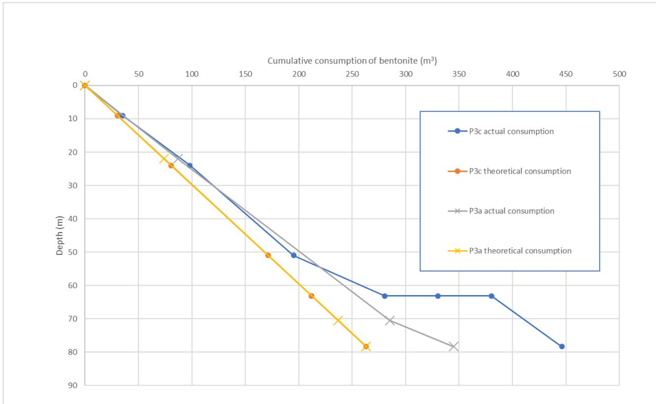
Figure 15 Cumulative consumption of bentonite vs. depth for bites 3a and 3c
