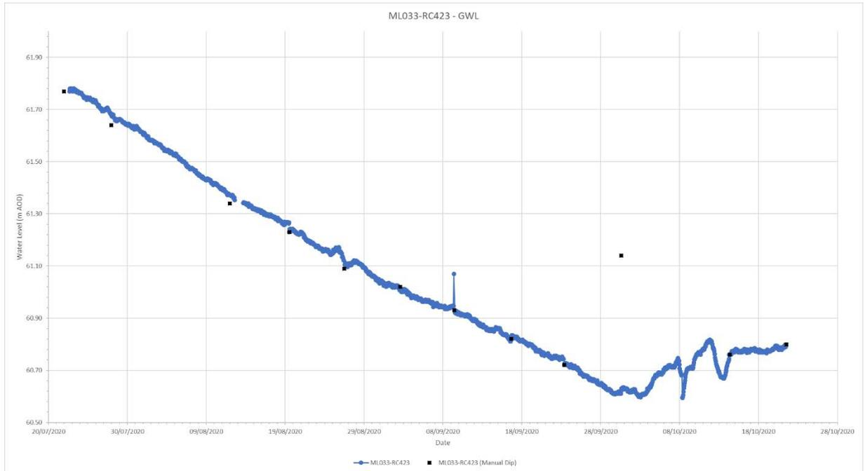
Figure 33 – Water level variations in RC423 during d-walling
