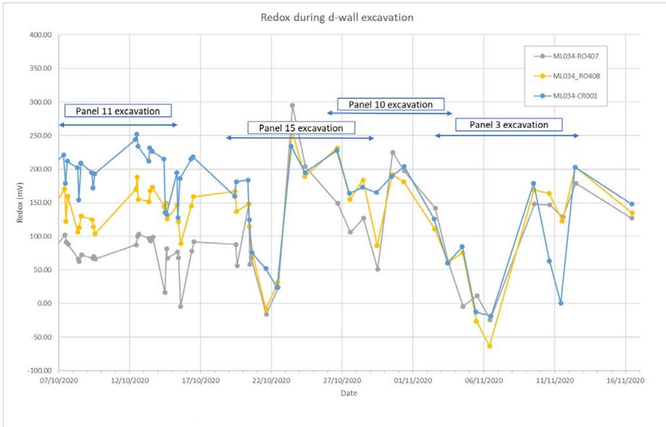
Figure 26 – Redox during excavation of Panels 11 to 3
