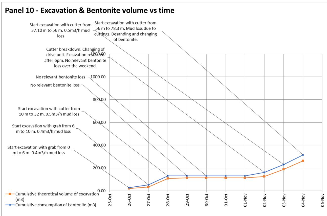
Figure 14 Cumulative consumption of bentonite vs. time for Panel 10
