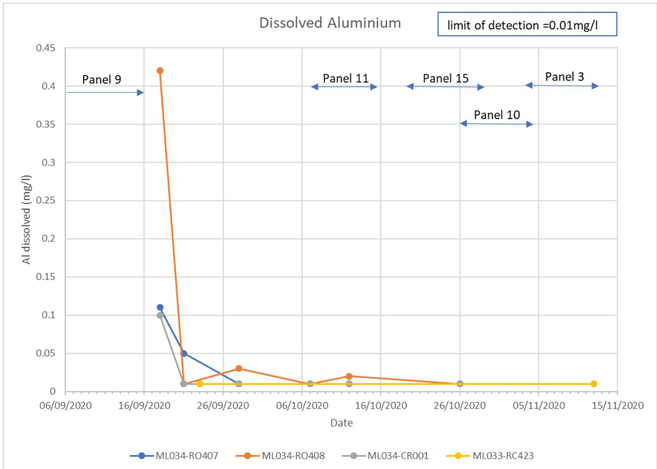
Figure 27 – Dissolved aluminium concentrations during d-walling
