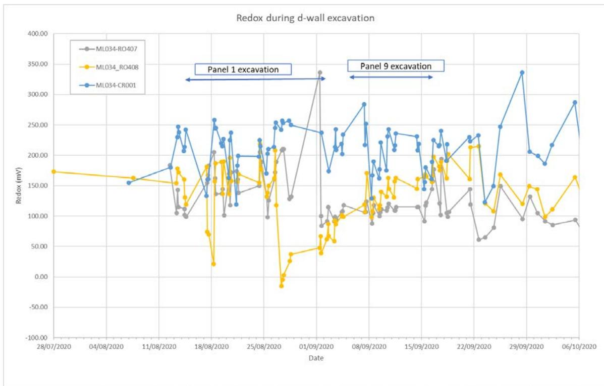
Figure 19 – Redox during d-wall excavation
