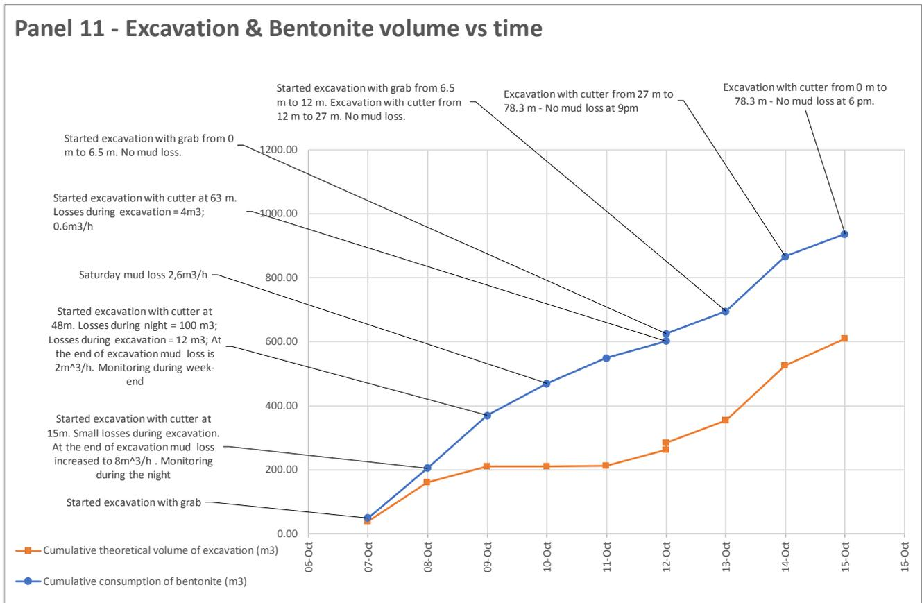
Figure 10 Cumulative consumption of bentonite vs. time for Panel 11
