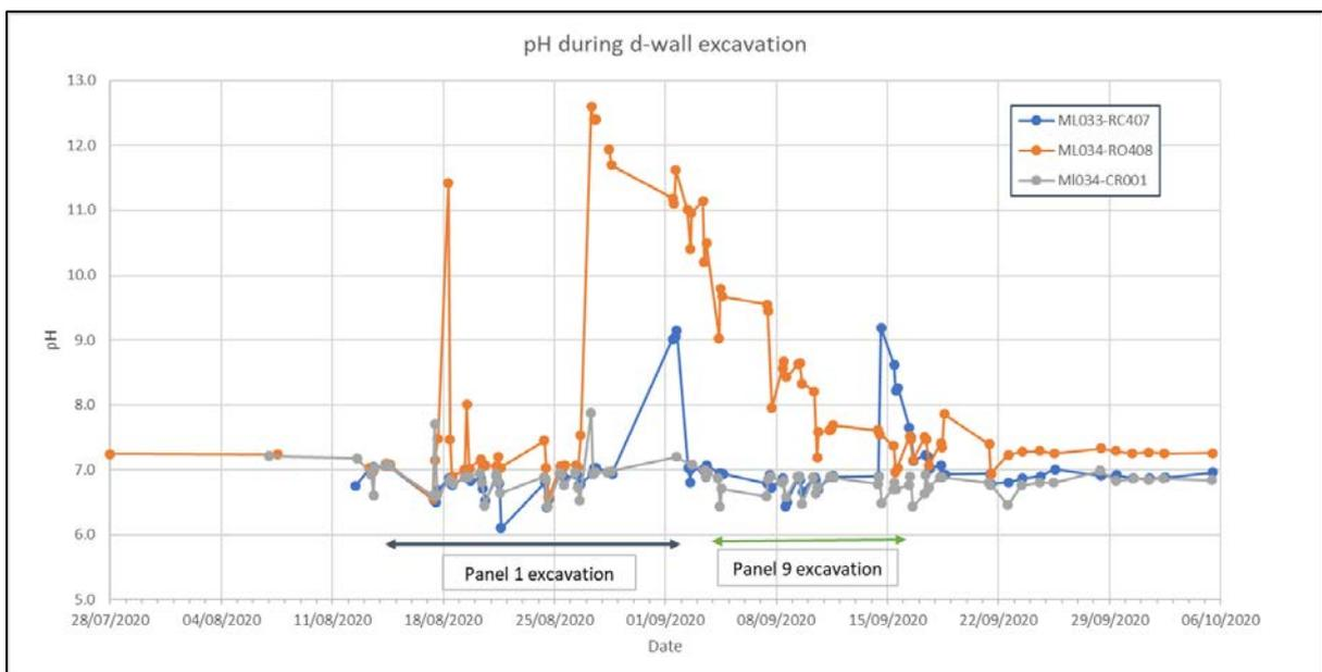
Figure 17 – pH during d-wall excavation of Panels 1 and 9
