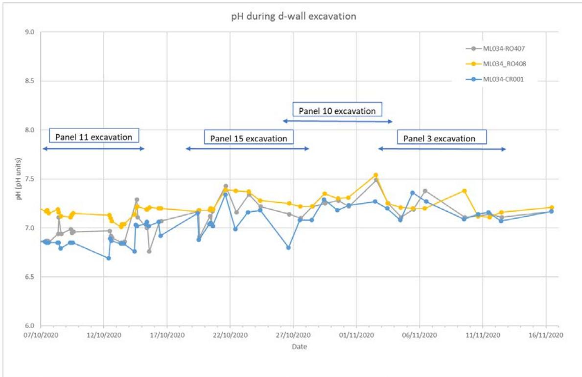
Figure 22 – pH during d-wall excavation of Panels 11 to 3
