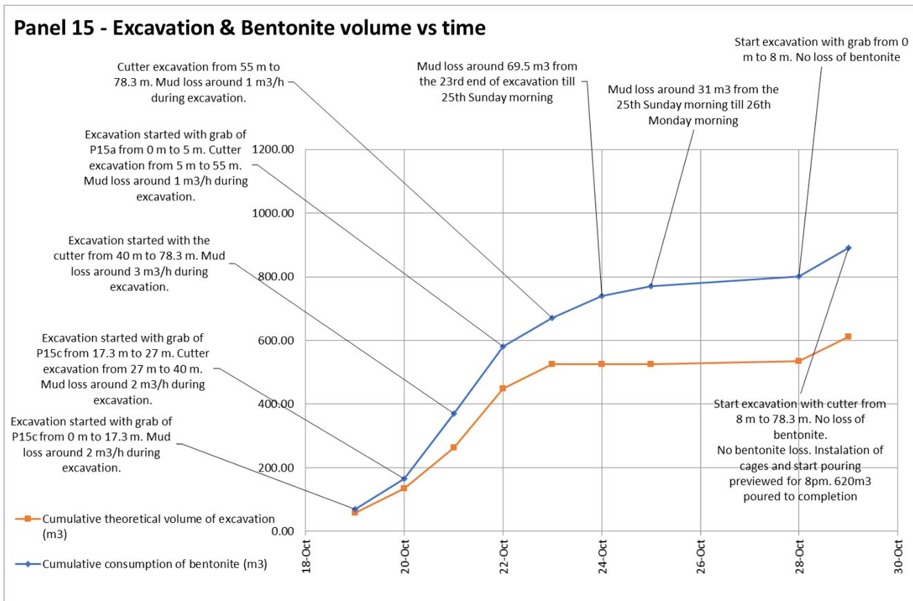
Figure 12 Cumulative consumption of bentonite vs. time for Panel 15
