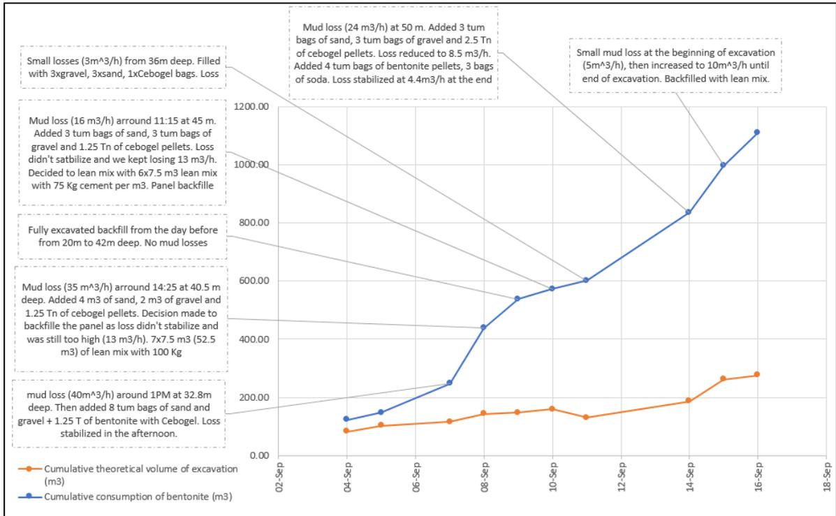
Figure 7 Cumulative consumption of bentonite vs. time for Panel 9
