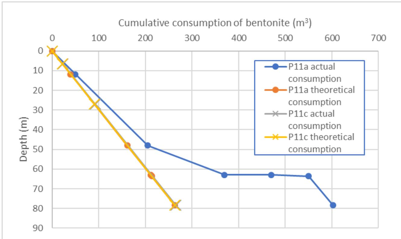
Figure 9 Cumulative consumption of bentonite vs. depth for Panels 11a and 11c
