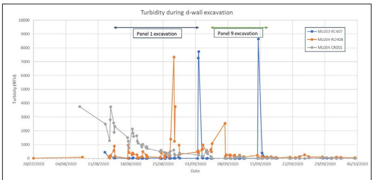
Figure 18 – turbidity during d-wall excavation
