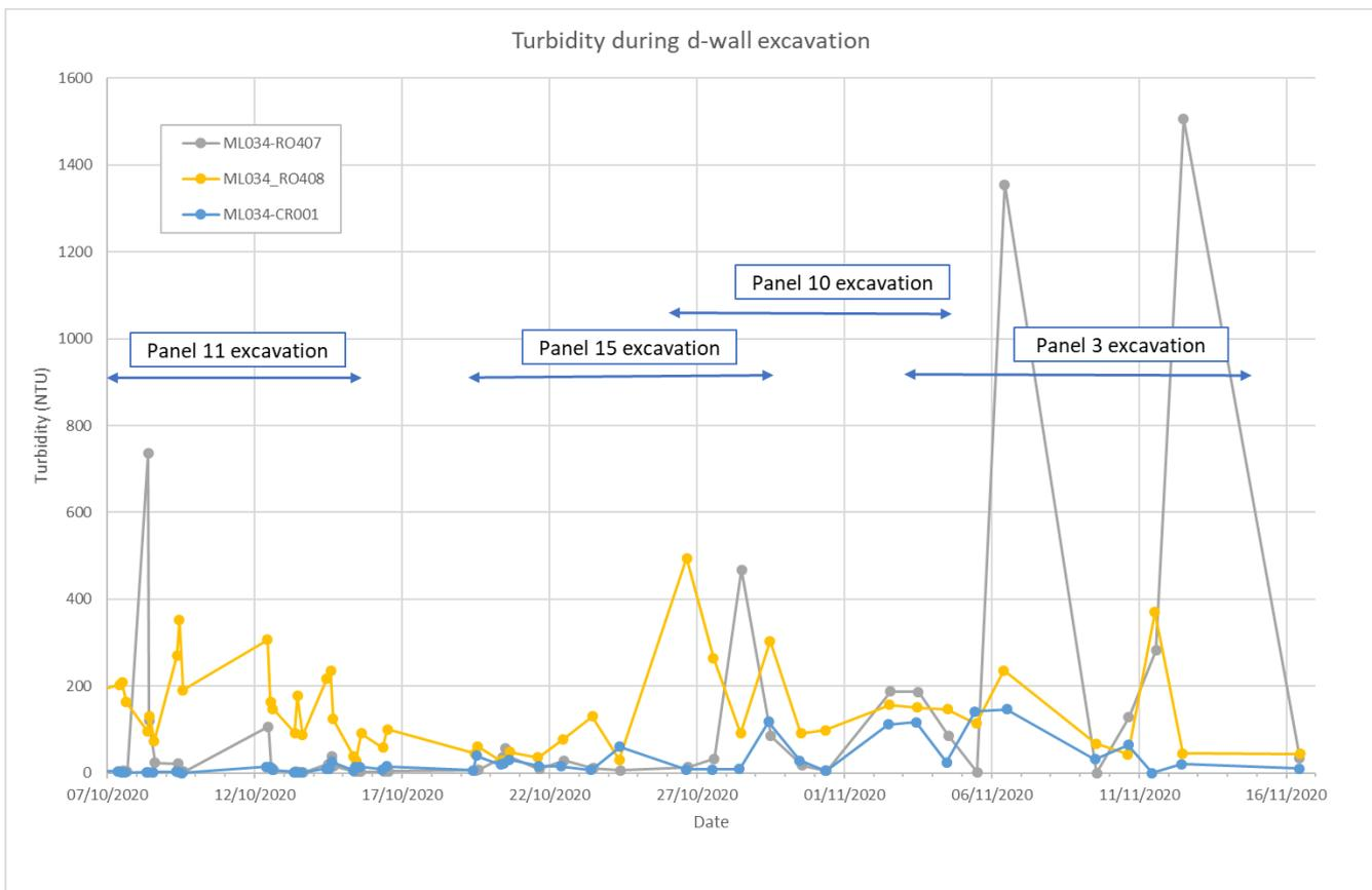
Figure 24 – Turbidity during excavation of Panels 11 to 3
