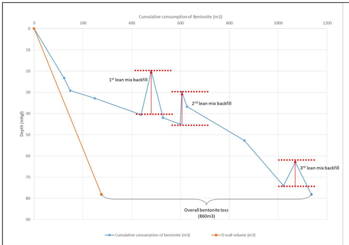
Figure 6 - Cumulative consumption of bentonite vs. depth for Panel 9
