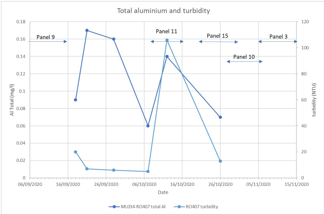
Figure 29 – Total aluminium versus turbidity at RO407
