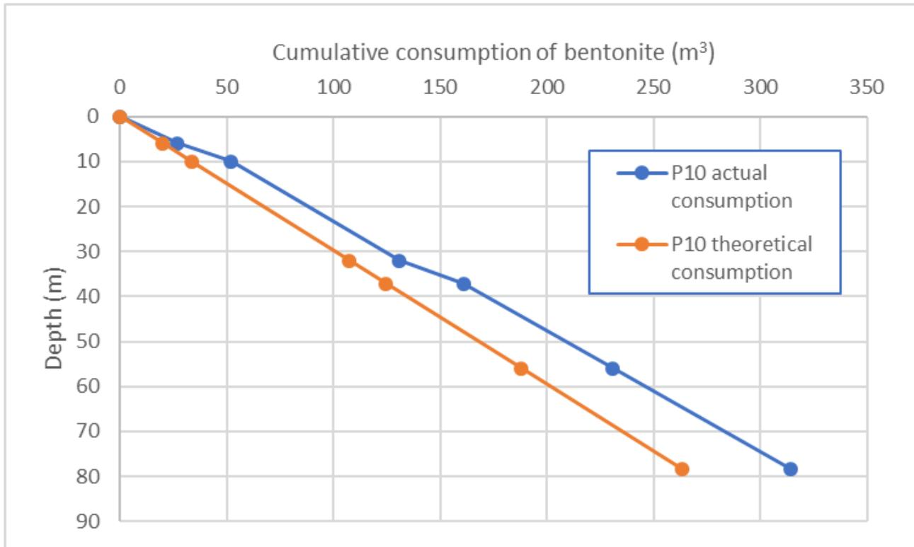
Figure 13 Cumulative consumption of bentonite vs. depth for Panel 10
