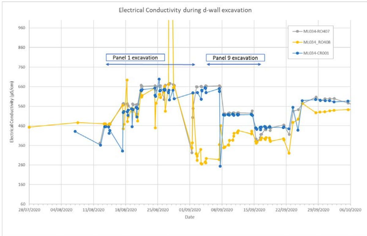
Figure 20 – Electrical conductivity during d-wall excavation
